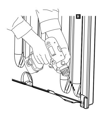
Align the lap joint between Front Right Side (H) and Repeat Right Side (E).
